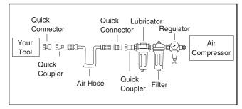
Figure 2. Installing your tool.
